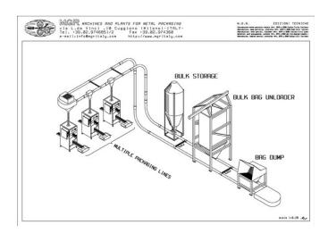
Cable transport system, designed to transport powders, flours, ground grains, grains gently and without breaking at the desired distance and height in the desired quantity.
