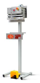
Vertical pneumatic welding machine with hot electrodes for heat sealable bags, with compressed air, with area for lot and date that can be easily updated.
